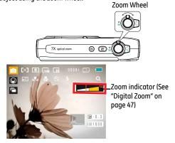
Optical zoom is initially used until it reaches the maximal threshold. Thereafter, it will switch over from optical to digital zoom. After adjusting, the zoom axis display will be hidden, only T  $\mathbf{Q}$  will be displayed to indicate the current zoom status.
